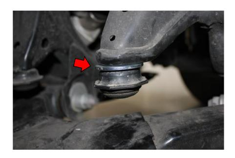
Install 1 bump stop spacer per side as shown
