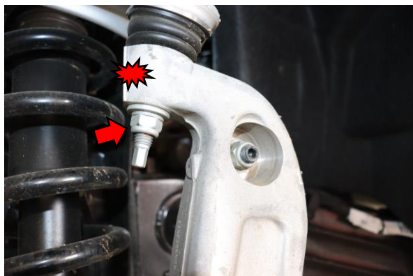
5. Loosen but do not remove 18mm upper ball joint nut. Use a hammer against the top of the steering knuckle to shock loose the upper ball joint.
