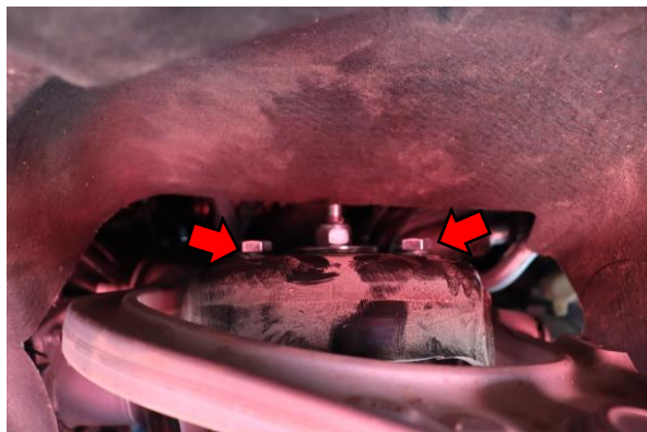
13. Use 17mm to install three top hat bolts and tighten to manufacturer specification.
