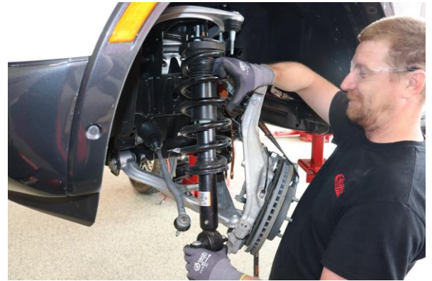
10. Remove the shock assembly from the vehicle.
