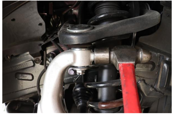
8. Use a hammer to shock loose the upper control arm ball joint and the outer tie rod end.
