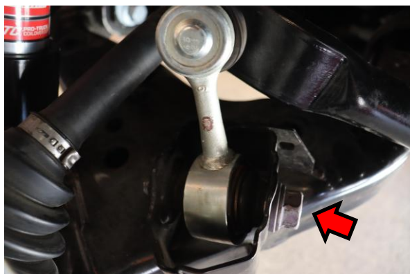
19. Install the sway bar end link bolt and tighten to manufacturer specification.
