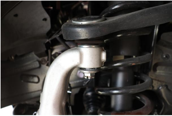
7. Loosen but do not remove the upper control arm ball joint nut.
