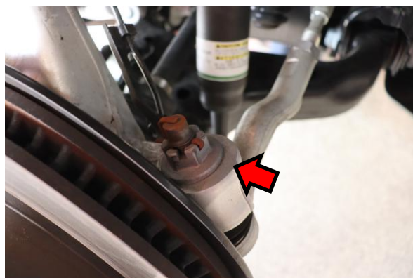
20. Install tie rod end nut and tighten to manufacturer specification.
