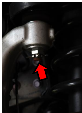
2. Remove cotter pins from the upper ball joint and outer tie rod end.
