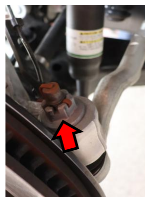
2. Remove cotter pins from the upper ball joint and outer tie rod end.
