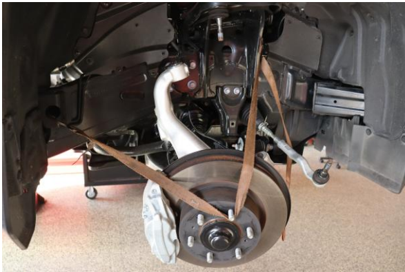
9. Use a strap to limit the spindle. This prevents damage to the axle from overextending.
