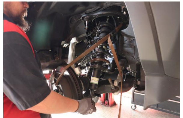
12. Slide the shock off the lower mount and lower the assembly out of the vehicle.
