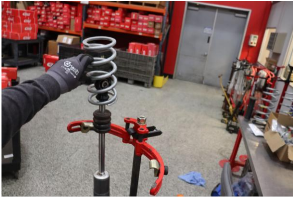
Step 13. Install Eibach secondary spring.
