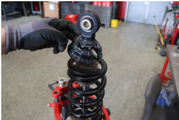
Step 7. Remove the spring retainer.
