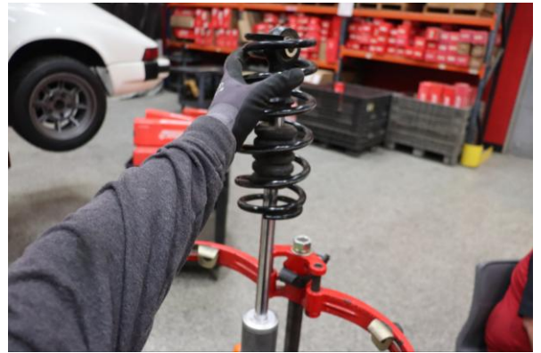
Step 10. Remove tender spring.
