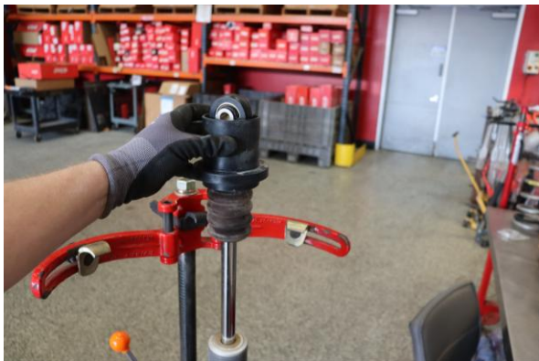
Step 9. Remove spring slider.
