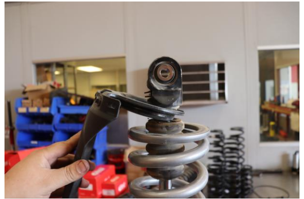
Step 16. Install lower spring retainer. Decompress spring assembly making sure that lower spring retainer and main spring sit flush with lower shock mount.
