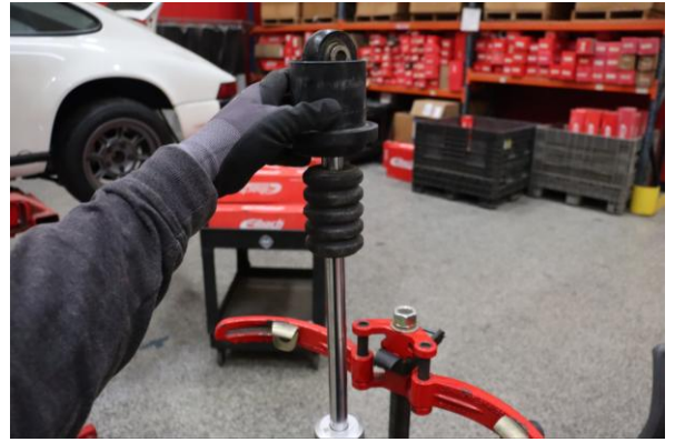
Step 8. Remove OE slider
