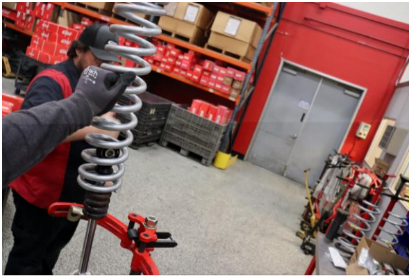
Step 15. Install Eibach main spring.
