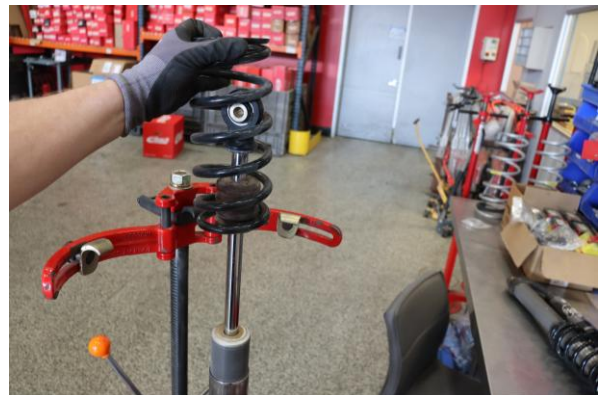
Step 10. Remove OE secondary spring.
