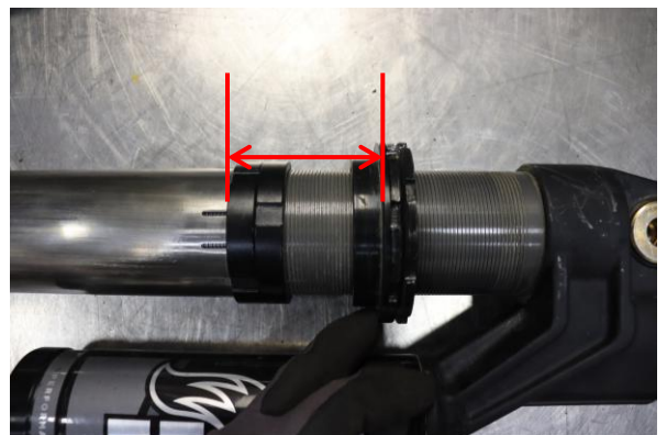
Step 12. Set crossover ring to 70mm (2 3/4in.) from bottom of spring seat to bottom of crossover ring.
